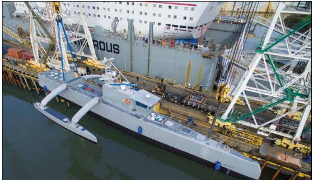
The Defense Advanced Research Projects Agency (DARPA)’s anti-submarine warfare continuous trail unmanned vessel (ACTUV) is a new class of unmanned ocean-going vessels able to travel thousands of miles over the open seas for months at a time, without a crew, and with a high degree of autonomy in operation. The ACTUV technology demonstrator was launched at its construction site in Portland, Oregon, on April 7, 2016.
