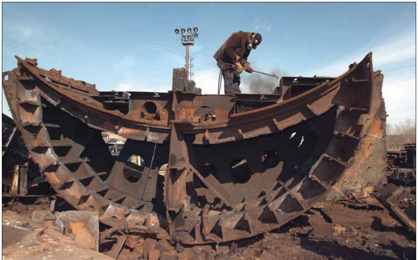
Torched. A Russian shipyard worker uses a cutting torch to break down a large bulge section of a Russian Oscar Class submarine at the Little Star shipyard in Severodvinsk, Russia, May 29, 1996. Russian ballistic submarines are being dismantled as part of the Nunn-Lugar/Cooperative Threat Reduction Program. (DoD photo by Petty Officer 1st Class Todd P. Cichonowicz, US Navy)
