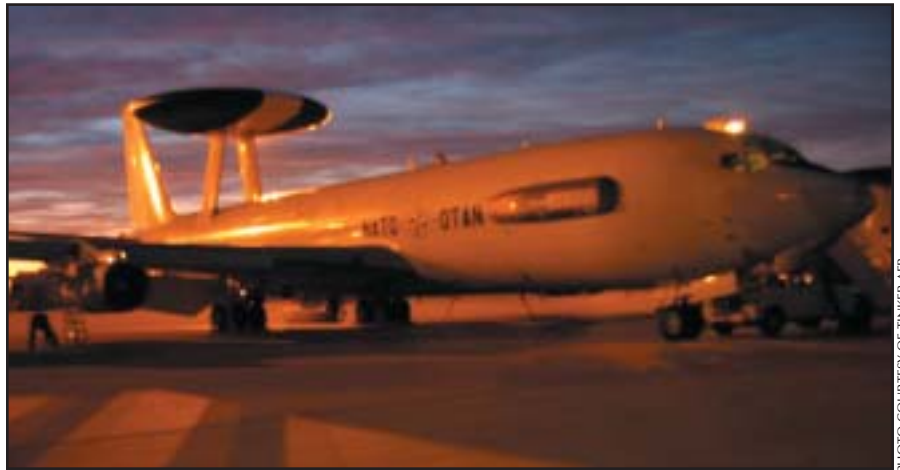
One of five NATO E-3A AWACS planes at Tinker Air Force Base in Oklahoma City. This plane is a modified Boeing 707 with a six-ton radar dome mounted on top. The jets carry no weaponry and refuel in mid-air.
